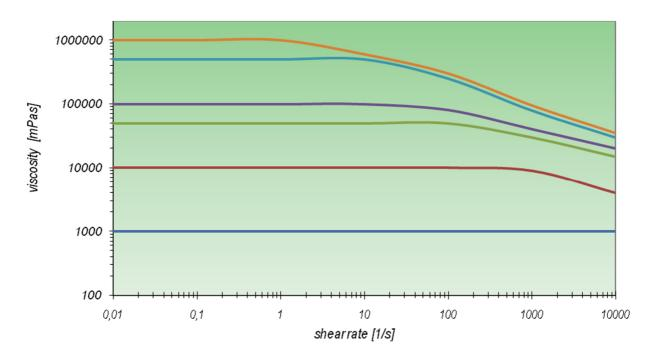
It can be seen in general, that with increasing viscosity of the **KORASILON**<sup>®</sup> **Fluid M** the *Newtonian area*, the interval where viscosity is independent from shear rate (indicated by the horizontal part of the curve) is decreasing, while shear thinning behaviour (viscosity is decreasing with increasing shear rate) is becoming more and more evident.
