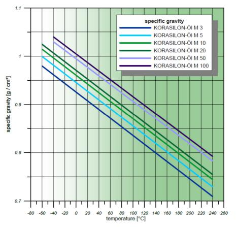
The temperature/specific-density curve of **KORASILON® Fluid M 100** is describing the temperature dependency of any **KORASILON® Fluid M** with viscosities higher than 100 mm<sup>2</sup>/s.
